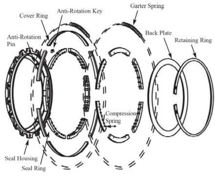
A combination of compression and garter springs ensures that the segments remain in contact with mating surfaces during low delta pressure and at shutdown conditions.
